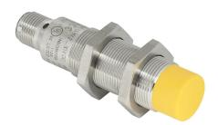
ifm efector inductive proximity sensor, tubular, 18mm diameter x 70.5mm body, stainless steel housing, PNP, (2) OSSD, 1-8mm enable zone, non-flush, IP65 IP67, 4-pin M12 quick-disconnect.
