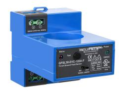
AcuAMP ground fault sensor, large aperture fixed core, 5, 10, or 30 mA selectable trip point, relay, SPDT normally de-energized, automatic reset output, 120 VAC operating voltage.
