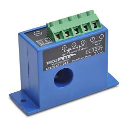
AcuAMP ground fault sensor, fixed core, 5, 10, or 30 mA selectable trip point, relay, SPDT normally energized, automatic reset output, 24 VAC/VDC operating voltage.
