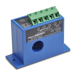
AcuAMP ground fault sensor, fixed core, 5, 10, or 30 mA selectable trip point, relay, SPDT normally de-energized, automatic reset output, 120 VAC operating voltage.
