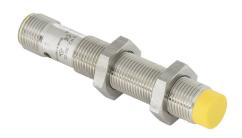
ifm efector inductive proximity sensor, tubular, 12mm diameter x 70mm body, stainless steel housing, PNP, (2) OSSD, 0.5-4mm enable zone, non-flush, IP65 IP67, 4-pin M12 quick-disconnect.
