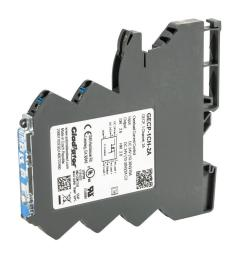
Gladiator electronic circuit protector, GECP series, 2A, 12/24 VDC, 1 channel(s), slow 1 curve, 35mm DIN rail mount.
