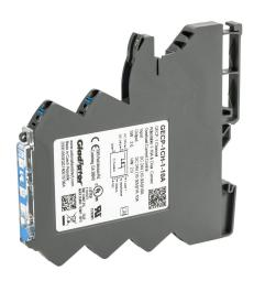
Gladiator electronic circuit protector, GECP series, adjustable 1-10A, 12/24 VDC, 1 channel(s), adjustable curve, 35mm DIN rail mount
