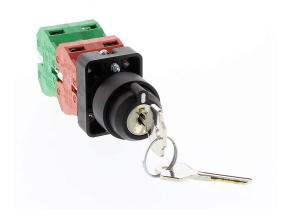
AutomationDirect selector switch, 22mm, 3-position, maintained, key removable in all positions, (2) N.O./(2) N.C. contact(s), plastic base, plastic bezel, Operator: black, key, 30mm, round, plastic.
