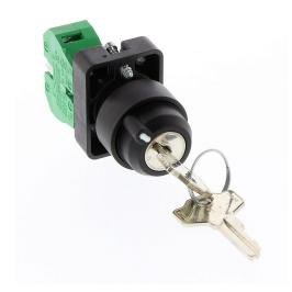
AutomationDirect selector switch, IP65, 22mm, 2-position, spring return from right, key removable left position, (1) N.O. contact(s), plastic base, plastic bezel, Operator: black, key, 30mm, round, plastic.
