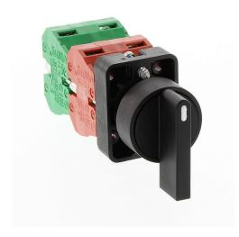
AutomationDirect selector switch, 22mm, 3-position, spring return to center, (2) N.O./(2) N.C. contact(s), plastic base, plastic bezel, Operator: black, lever, 30mm, round, plastic.
