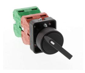
AutomationDirect selector switch, 22mm, 3-position, maintained, (2) N.O./(2) N.C. contact(s), plastic base, plastic bezel, Operator: black, lever, 30mm, round, plastic.
