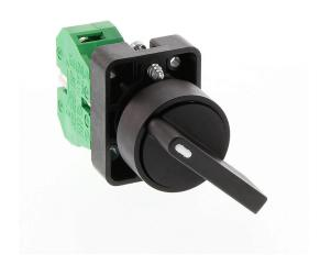
AutomationDirect selector switch, 22mm, 2-position, spring return from right, (1) N.O. contact(s), plastic base, plastic bezel, Operator: black, lever, 30mm, round, plastic.
