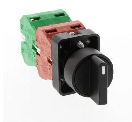
AutomationDirect selector switch, 22mm, 3-position, spring return to center, (2) N.O./(2) N.C. contact(s), plastic base, plastic bezel, Operator: black, knob, 30mm, round, plastic.
