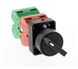
AutomationDirect selector switch, 22mm, 3-position, maintained, (2) N.O./(2) N.C. contact(s), plastic base, plastic bezel, Operator: black, knob, 30mm, round, plastic.
