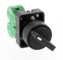
AutomationDirect selector switch, 22mm, 2-position, spring return from right, (1) N.O. contact(s), plastic base, plastic bezel, Operator: black, knob, 30mm, round, plastic.
