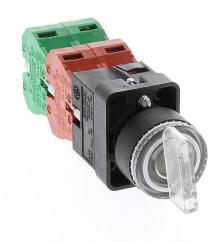
AutomationDirect selector switch, 22mm, 3-position, spring return to center, incandescent illuminated, (2) N.O./(2) N.C. contact(s), plastic base, plastic bezel, Operator: clear, knob, 30mm, round, plastic, 24 VAC/VDC, full voltage.
