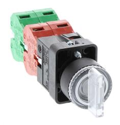
AutomationDirect selector switch, 22mm, 3-position, spring return to center, LED illuminated, (2) N.O./(2) N.C. contact(s), plastic base, plastic bezel, Operator: clear, knob, 30mm, round, plastic, 24 VAC/VDC, full voltage.
