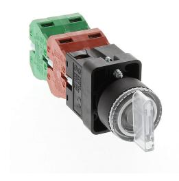
AutomationDirect selector switch, 22mm, 3-position, spring return to center, incandescent illuminated, (2) N.O./(2) N.C. contact(s), plastic base, plastic bezel, Operator: clear, knob, 30mm, round, plastic, 120 VAC/VDC, full voltage.
