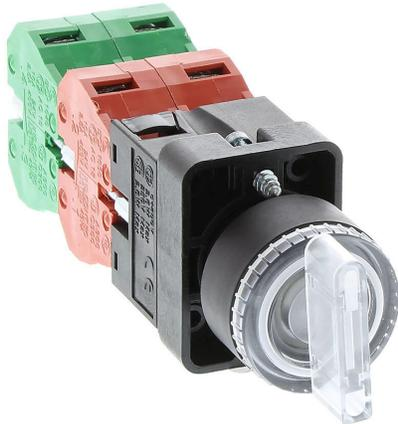
AutomationDirect selector switch, 22mm, 3-position, spring return to center, LED illuminated, (2) N.O./ (2) N.C. contact(s), plastic base, plastic bezel, Operator: clear, knob, 30mm, round, plastic, 120 VAC/VDC, full voltage.
