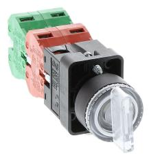
AutomationDirect selector switch, 22mm, 3-position, spring return to center, LED illuminated, (2) N.O./(2) N.C. contact(s), plastic base, plastic bezel, Operator: clear, knob, 30mm, round, plastic, 120 VAC/VDC, full voltage.
