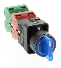
AutomationDirect selector switch, 22mm, 3-position, spring return to center, incandescent illuminated, (2) N.O./(2) N.C. contact(s), plastic base, plastic bezel, Operator: blue, knob, 30mm, round, plastic, 24 VAC/VDC, full voltage.
