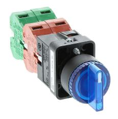
AutomationDirect selector switch, 22mm, 3-position, spring return to center, LED illuminated, (2) N.O./(2) N.C. contact(s), plastic base, plastic bezel, Operator: blue, knob, 30mm, round, plastic, 24 VAC/VDC, full voltage.
