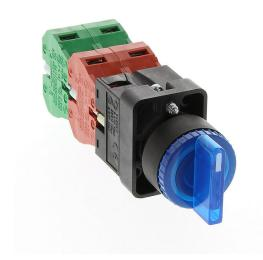
AutomationDirect selector switch, 22mm, 3-position, spring return to center, incandescent illuminated, (2) N.O./(2) N.C. contact(s), plastic base, plastic bezel, Operator: blue, knob, 30mm, round, plastic, 120 VAC/VDC, full voltage.
