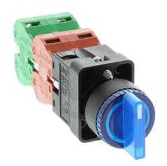
AutomationDirect selector switch, 22mm, 3-position, spring return to center, LED illuminated, (2) N.O./(2) N.C. contact(s), plastic base, plastic bezel, Operator: blue, knob, 30mm, round, plastic, 120 VAC/VDC, full voltage.
