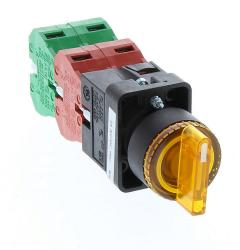
AutomationDirect selector switch, 22mm, 3-position, spring return to center, incandescent illuminated, (2) N.O./(2) N.C. contact(s), plastic base, plastic bezel, Operator: yellow, knob, 30mm, round, plastic, 24 VAC/VDC, full voltage.
