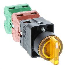
AutomationDirect selector switch, 22mm, 3-position, spring return to center, LED illuminated, (2) N.O./(2) N.C. contact(s), plastic base, plastic bezel, Operator: yellow, knob, 30mm, round, plastic, 24 VAC/VDC, full voltage.
