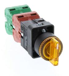
AutomationDirect selector switch, 22mm, 3-position, spring return to center, incandescent illuminated, (2) N.O./(2) N.C. contact(s), plastic base, plastic bezel, Operator: yellow, knob, 30mm, round, plastic, 120 VAC/VDC, full voltage.
