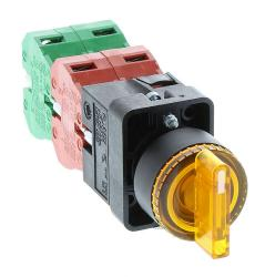
AutomationDirect selector switch, 22mm, 3-position, spring return to center, LED illuminated, (2) N.O./(2) N.C. contact(s), plastic base, plastic bezel, Operator: yellow, knob, 30mm, round, plastic, 120 VAC/VDC, full voltage.
