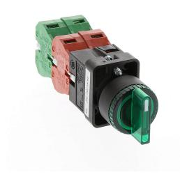
AutomationDirect selector switch, 22mm, 3-position, spring return to center, incandescent illuminated, (2) N.O./(2) N.C. contact(s), plastic base, plastic bezel, Operator: green, knob, 30mm, round, plastic, 24 VAC/VDC, full voltage.
