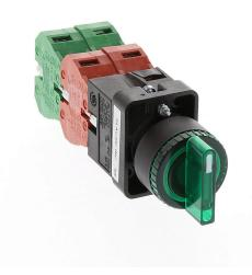
AutomationDirect selector switch, 22mm, 3-position, spring return to center, incandescent illuminated, (2) N.O./(2) N.C. contact(s), plastic base, plastic bezel, Operator: green, knob, 30mm, round, plastic, 24 VAC/VDC, full voltage.
