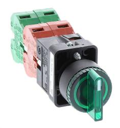
AutomationDirect selector switch, 22mm, 3-position, spring return to center, LED illuminated, (2) N.O./(2) N.C. contact(s), plastic base, plastic bezel, Operator: green, knob, 30mm, round, plastic, 24 VAC/VDC, full voltage.
