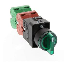
AutomationDirect selector switch, 22mm, 3-position, spring return to center, incandescent illuminated, (2) N.O./(2) N.C. contact(s), plastic base, plastic bezel, Operator: green, knob, 30mm, round, plastic, 120 VAC/VDC, full voltage.
