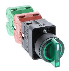
AutomationDirect selector switch, 22mm, 3-position, spring return to center, LED illuminated, (2) N.O./(2) N.C. contact(s), plastic base, plastic bezel, Operator: green, knob, 30mm, round, plastic, 120 VAC/VDC, full voltage.
