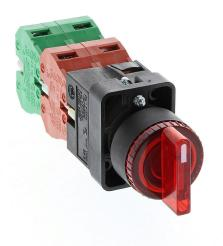
AutomationDirect selector switch, 22mm, 3-position, spring return to center, incandescent illuminated, (2) N.O./(2) N.C. contact(s), plastic base, plastic bezel, Operator: red, knob, 30mm, round, plastic, 24 VAC/VDC, full voltage.
