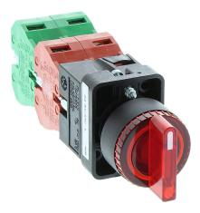
AutomationDirect selector switch, 22mm, 3-position, spring return to center, LED illuminated, (2) N.O./(2) N.C. contact(s), plastic base, plastic bezel, Operator: red, knob, 30mm, round, plastic, 24 VAC/VDC, full voltage.
