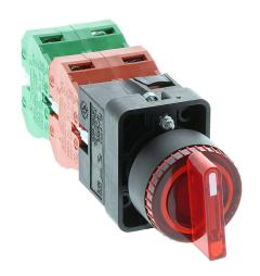
AutomationDirect selector switch, 22mm, 3-position, spring return to center, incandescent illuminated, (2) N.O./(2) N.C. contact(s), plastic base, plastic bezel, Operator: red, knob, 30mm, round, plastic, 120 VAC/VDC, full voltage.
