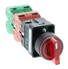
AutomationDirect selector switch, 22mm, 3-position, spring return to center, LED illuminated, (2) N.O./(2) N.C. contact(s), plastic base, plastic bezel, Operator: red, knob, 30mm, round, plastic, 120 VAC/VDC, full voltage.
