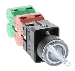
AutomationDirect selector switch, 22mm, 3-position, maintained, LED illuminated, (2) N.O./(2) N.C. contact(s), plastic base, plastic bezel, Operator: clear, knob, 30mm, round, plastic, 24 VAC/VDC, full voltage.
