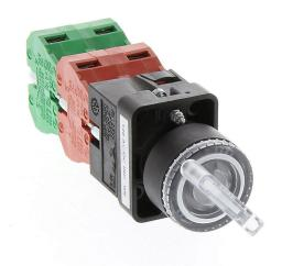
AutomationDirect selector switch, 22mm, 3-position, maintained, incandescent illuminated, (2) N.O./(2) N.C. contact(s), plastic base, plastic bezel, Operator: clear, knob, 30mm, round, plastic, 120 VAC/VDC, full voltage.
