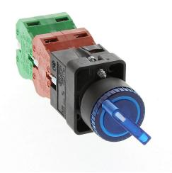
AutomationDirect selector switch, 22mm, 3-position, maintained, incandescent illuminated, (2) N.O./(2) N.C. contact(s), plastic base, plastic bezel, Operator: blue, knob, 30mm, round, plastic, 24 VAC/VDC, full voltage.
