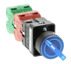
AutomationDirect selector switch, 22mm, 3-position, maintained, LED illuminated, (2) N.O./(2) N.C. contact(s), plastic base, plastic bezel, Operator: blue, knob, 30mm, round, plastic, 24 VAC/VDC, full voltage.
