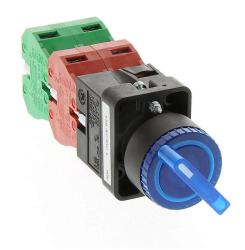
AutomationDirect selector switch, 22mm, 3-position, maintained, incandescent illuminated, (2) N.O./(2) N.C. contact(s), plastic base, plastic bezel, Operator: blue, knob, 30mm, round, plastic, 120 VAC/VDC, full voltage.
