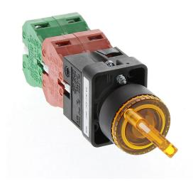
AutomationDirect selector switch, 22mm, 3-position, maintained, incandescent illuminated, (2) N.O./(2) N.C. contact(s), plastic base, plastic bezel, Operator: yellow, knob, 30mm, round, plastic, 24 VAC/VDC, full voltage.
