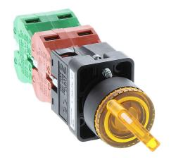
AutomationDirect selector switch, 22mm, 3-position, maintained, LED illuminated, (2) N.O./(2) N.C. contact(s), plastic base, plastic bezel, Operator: yellow, knob, 30mm, round, plastic, 24 VAC/VDC, full voltage.
