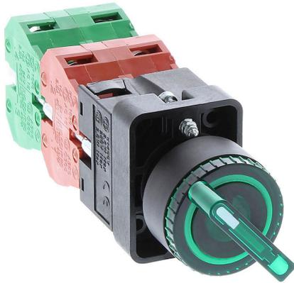
AutomationDirect selector switch, 22mm, 3-position, maintained, LED illuminated, (2) N.O./ (2) N.C. contact(s), plastic base, plastic bezel, Operator: green, knob, 30mm, round, plastic, 24 VAC/VDC, full voltage.
