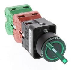
AutomationDirect selector switch, 22mm, 3-position, maintained, incandescent illuminated, (2) N.O./(2) N.C. contact(s), plastic base, plastic bezel, Operator: green, knob, 30mm, round, plastic, 120 VAC/VDC, full voltage.
