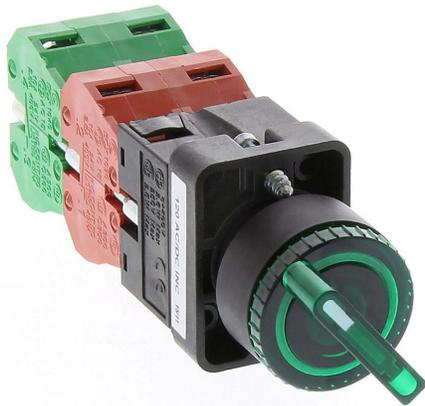
AutomationDirect selector switch, 22mm, 3-position, maintained, incandescent illuminated, (2) N.O./ (2) N.C. contact(s), plastic base, plastic bezel, Operator: green, knob, 30mm, round, plastic, 120 VAC/VDC, full voltage.
