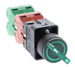
AutomationDirect selector switch, 22mm, 3-position, maintained, LED illuminated, (2) N.O./(2) N.C. contact(s), plastic base, plastic bezel, Operator: green, knob, 30mm, round, plastic, 120 VAC/VDC, full voltage.
