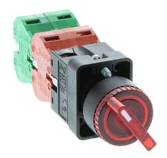
AutomationDirect selector switch, 22mm, 3-position, maintained, LED illuminated, (2) N.O./(2) N.C. contact(s), plastic base, plastic bezel, Operator: red, knob, 30mm, round, plastic, 24 VAC/VDC, full voltage.
