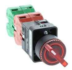
AutomationDirect selector switch, 22mm, 3-position, maintained, LED illuminated, (2) N.O./(2) N.C. contact(s), plastic base, plastic bezel, Operator: red, knob, 30mm, round, plastic, 120 VAC/VDC, full voltage.
