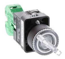
AutomationDirect selector switch, 22mm, 2-position, maintained, LED illuminated, (1) N.O. contact(s), plastic base, plastic bezel, Operator: clear, knob, 30mm, round, plastic, 120 VAC/VDC, full voltage.
