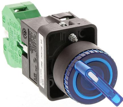
AutomationDirect selector switch, 22mm, 2-position, maintained, incandescent illuminated, (1) N.O. contact(s), plastic base, plastic bezel, Operator: blue, knob, 30mm, round, plastic, 24 VAC/VDC, full voltage.
