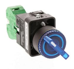
AutomationDirect selector switch, 22mm, 2-position, maintained, incandescent illuminated, (1) N.O. contact(s), plastic base, plastic bezel, Operator: blue, knob, 30mm, round, plastic, 24 VAC/VDC, full voltage.
