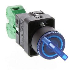
AutomationDirect selector switch, 22mm, 2-position, maintained, LED illuminated, (1) N.O. contact(s), plastic base, plastic bezel, Operator: blue, knob, 30mm, round, plastic, 24 VAC/VDC, full voltage.
